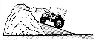
Another method for large dirt piles is to build a ramp approach to the pile.
